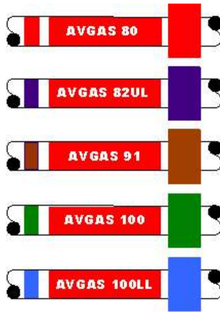
Figure 1: Aviation gasoline identification band, label and colour coding
